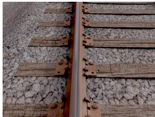
B: Over-the-rail view showing both sides of the simulated tie plate and crib ballast
